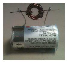
7. Place a neodymium magnet onto the C battery and directly under the center of your coil. The setup should look like the image below.
