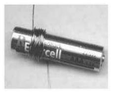
2. Carefully pull the coil off the form, holding the wire so it doesn't spring out of shape. To make the coil hold its shape, wrap each free end of the wire around the coil a couple of times. Make sure the new
