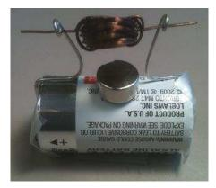
8. Gently give your coil a spin. You may have to try spinning it either direction – the coil will only spin in one direction. If everything is well-aligned, your coil should begin spinning continuously.
